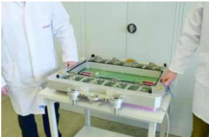
Figure 2: Twinning Frame with MultiLane BERTs, DSOs, and AWGs inside.
